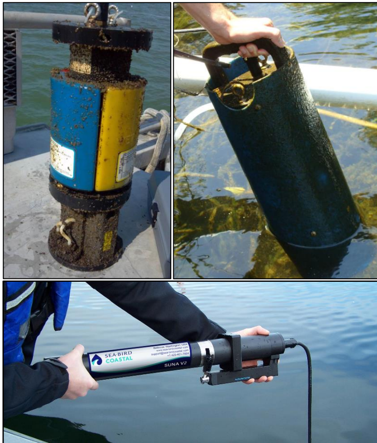
Figure 2-7. These Sea-Bird Coastal Cycle PO 4 phosphate sensors have accumulated an external bio-fouling coating during deployment (top). A Satlantic SUNA nitrate sensor uses a rotating, motorized brush to keep the optical lenses free of bio-fouling. (Photos courtesy of Corey Koch/WET Labs)
