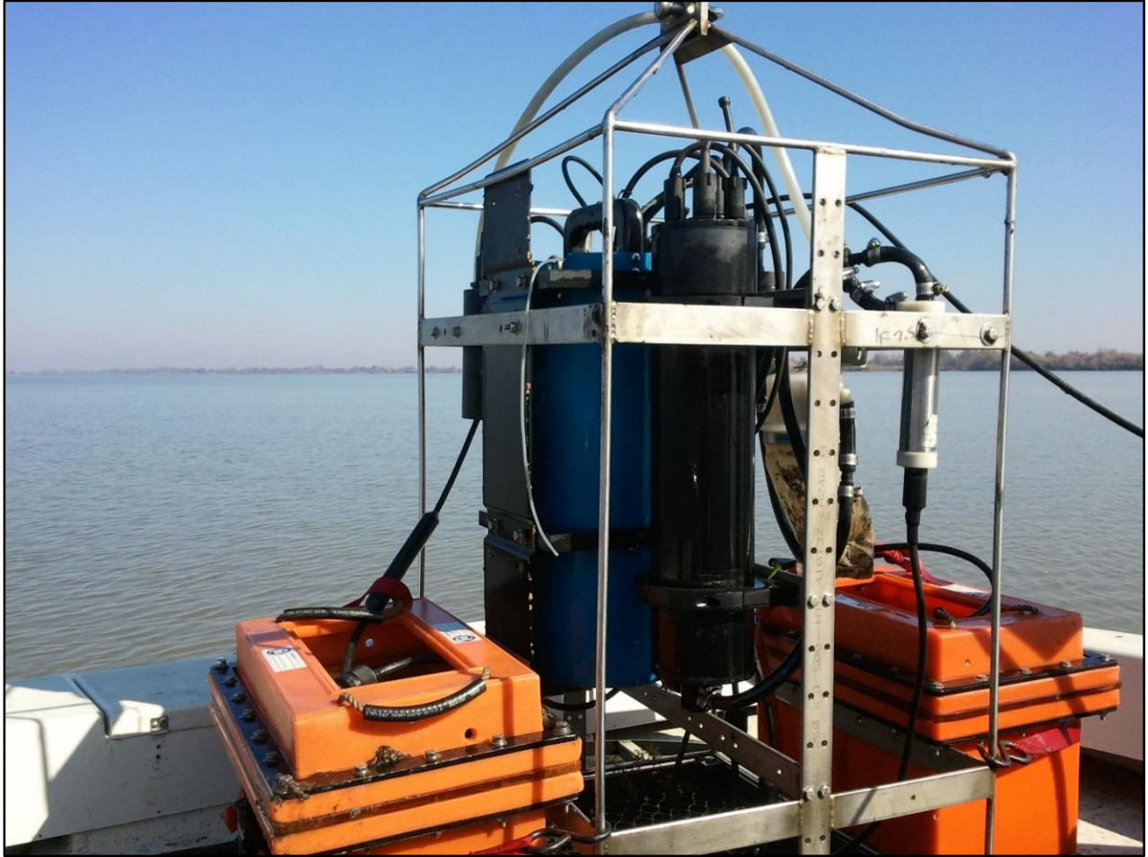
Figure 2-3. A cage for a boat deployment in the Bay Delta with several instruments (fluorometers, nitrate sensors, phosphate sensors, etc.). (Photo courtesy of Brian Pellerin/USGS)
